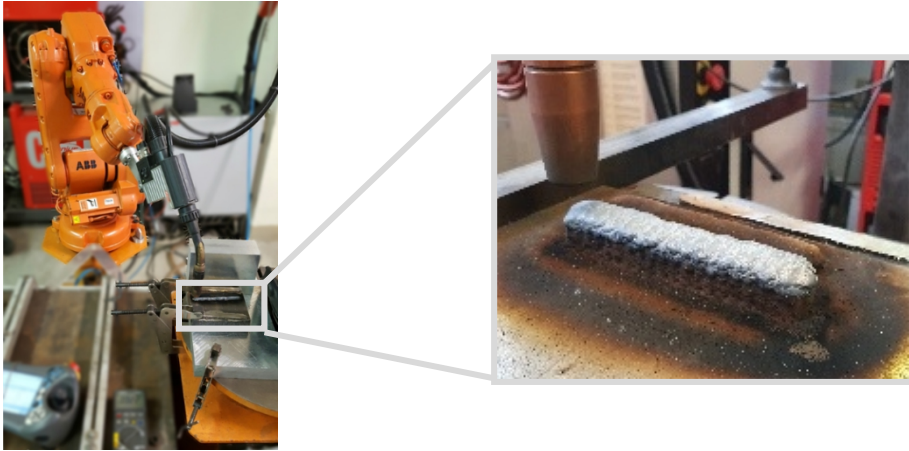
Figure 1. Experimental setup for the WAAM deposition process.
