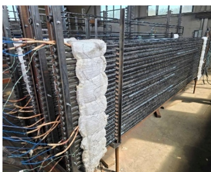
Figure 1. PWHT of X10CrMoVNb9-1 and 10CrMo9-10
