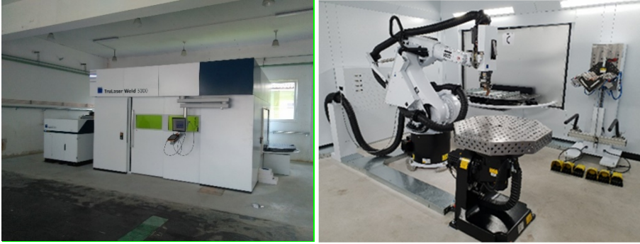
Figure 1. The laser robotic cell TruLaser Weld 5000
